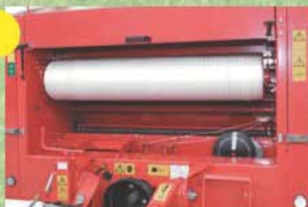
Ganci chiusura apertura portellone Hooks opening/closing rear door Crochets fermeture porte Haken Schließung/Öffnung/ Heckklappe Ganchos cierre abertura puerta
