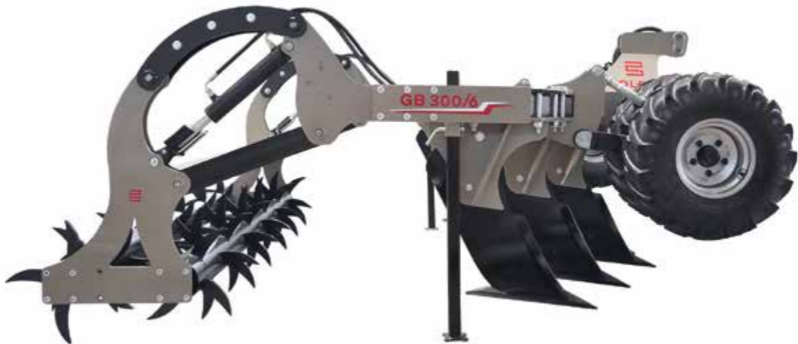
double Spiny roller with hydraulic adjustment
