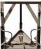
2 actuator under the hydropack
