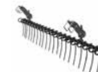
row of scrapers before/behind the roller
