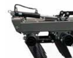
hydraulic adjustment of the harrow springs
