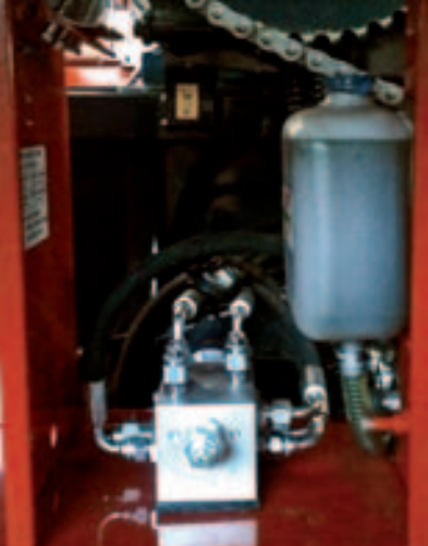
Valve unit to maintain pressure in the hydraulic circuit.
