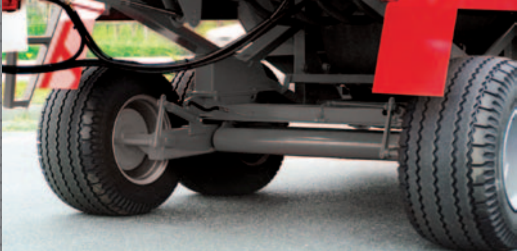
Double axle balance system tires 19.0/45-17 and hydraulic brake.
