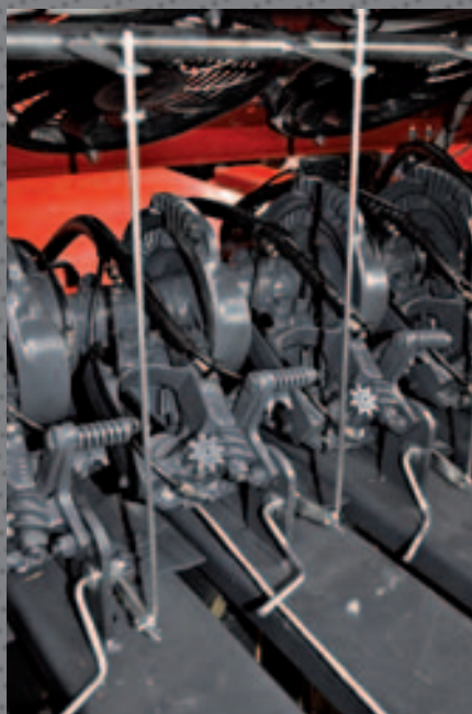
Binding anomaly detector with warning in cabin.
