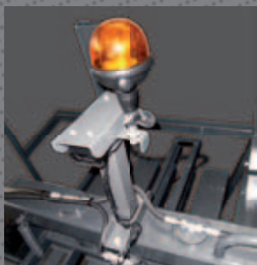
Two cameras, one for the view of knotters and one for the view of unloading ramp or bales stacker.
